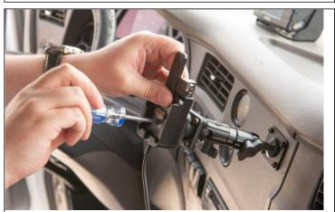
4. Re-attach the dock using the center screw. Tighten semi firmly and adjust the dock to the desired viewing position facing the driver. Then tighten the center screw firmly to lock the position.
