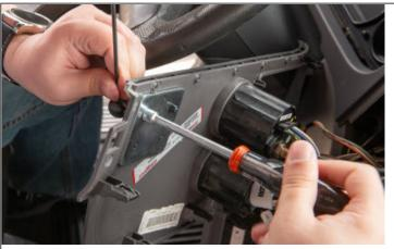
2. Line up the pedestal and the backing plate with the drilled holes. Secure in place using the enclosed screws and locking nuts.
